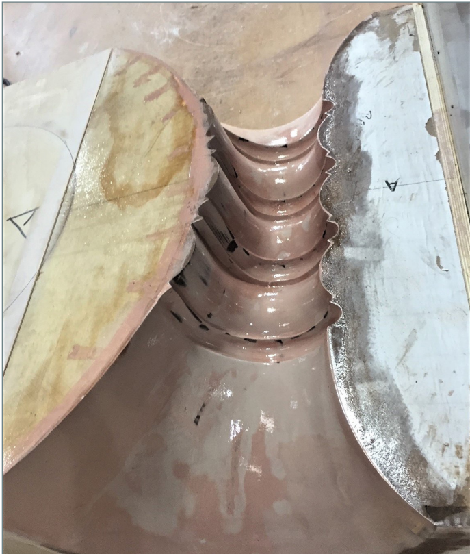
Lucas Concrete Products often combines wood, bonding putty and foam to make a mold. Photo courtesy of Lucas Concrete Products
