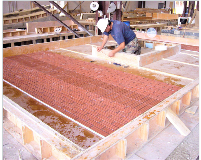
Architectural precast panels are made with form liners in a climate-controlled facility. Photo courtesy of American Stone Virginia
