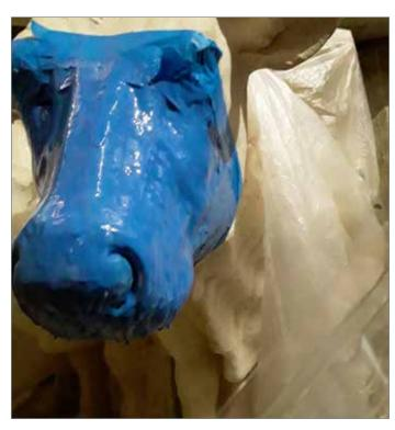
Step 3 – Create a two-part mold shell using a polyurethane plastic/liquid plastic. Brush apply the liquid plastic. We used a thin waffle board to create the seam between the left and right halves, be sure to create a raised flange on the waffle board to be able to create future bolt holes. We also incorporated a plastic conduit to create a pour hole for the repair material.
