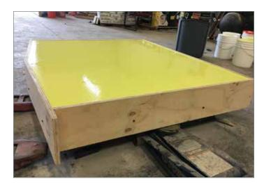
Step 4 – Remove the form work and strip the rubber molds.
